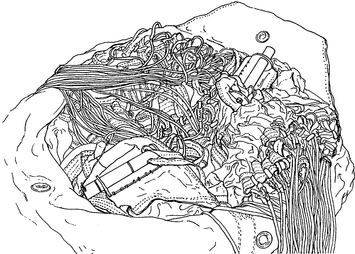
Figure 2-36. Canopy Stowing Completed.
