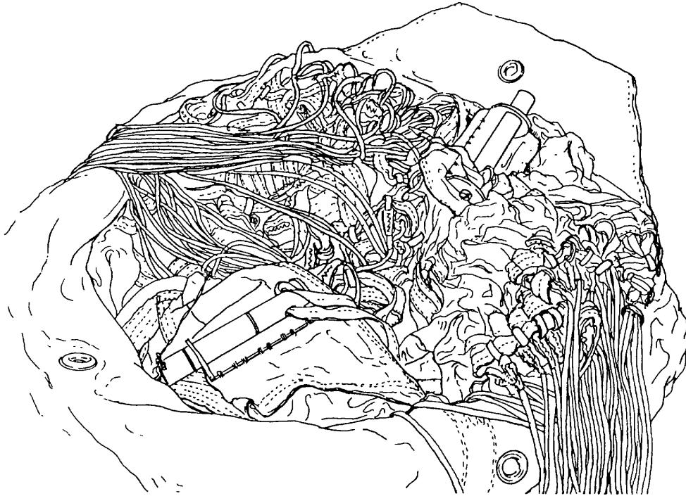
Figure 2-91. Canopy Stowed in Deployment Bag.
