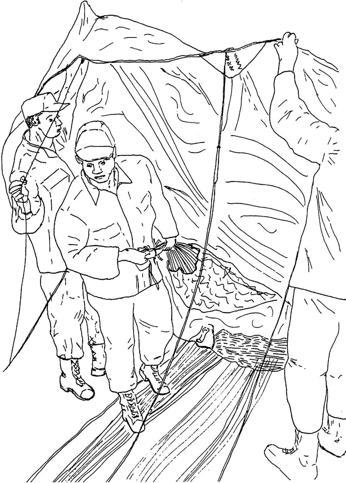
Figure 2-63. Removing Canopy Inversion.
