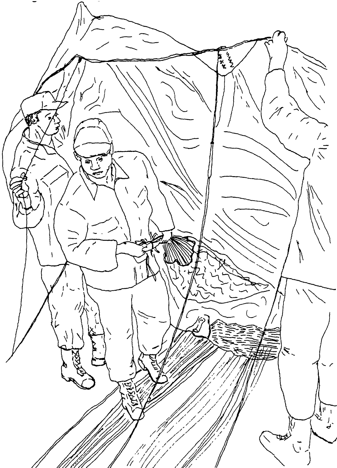
Figure 2-10. Removing Canopy Inversion.
