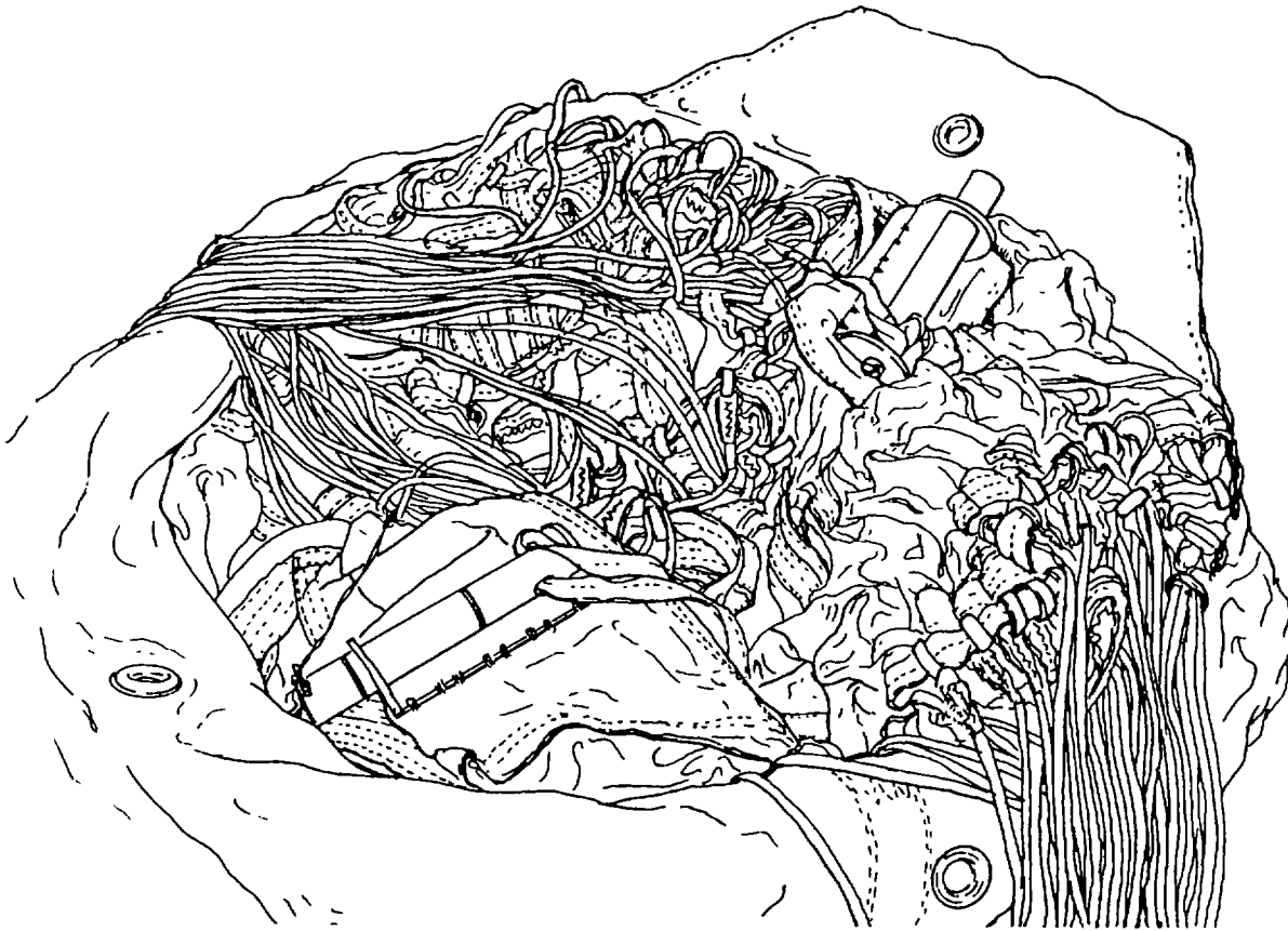
Figure 2-146. Canopy Stowed in Deployment Bag.
