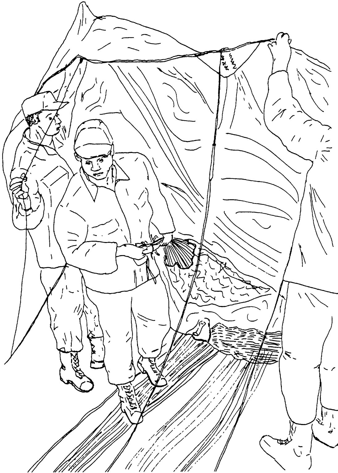
Figure 2-120. Removing Canopy Inversion.
